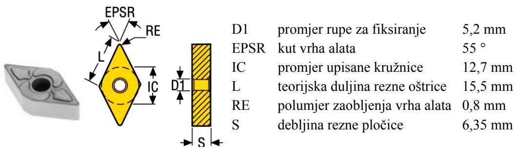
**Slika 5.4.** SECO rezna pločica DNMG 150608-MF-4 TP 2501 ([www.secotools.com](http://www.secotools.com))
