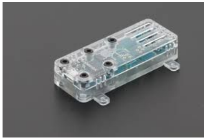
(c) Environmental sensor: Yoctopuce Yocto-Meteo-V2.
