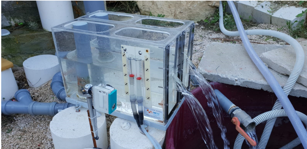
FIGURE A.18: V-Notch weirs for discharge measurement.
