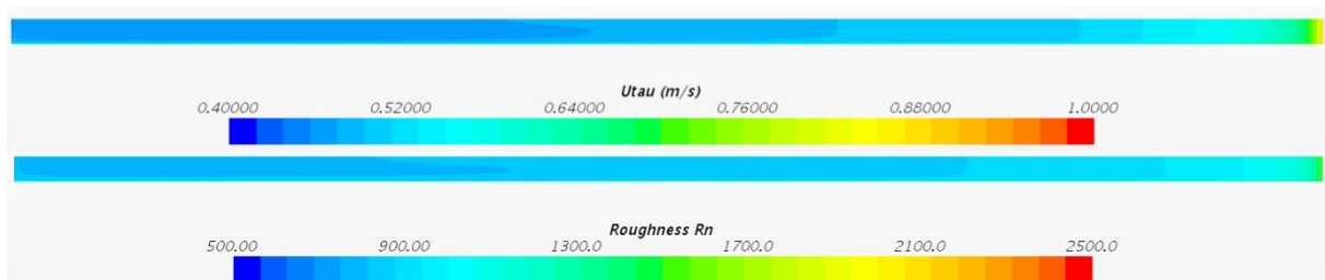
Figure 5.7 The obtained u_\tau distribution (upper) and k^+ distribution (lower) for the flat plate representing KCS, R1 H
