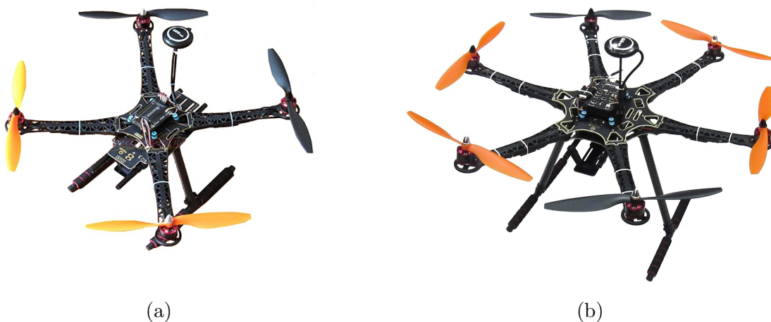
Figure 2.1: Multirotor types: quadrotor [89] (a), hexarotor [90] (b)
