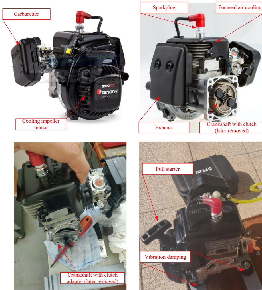
Figure 4.2: Photographs of Zenoah G320RC engines
