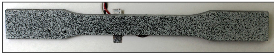
(a) Speckle pattern on the dog-bone sample
