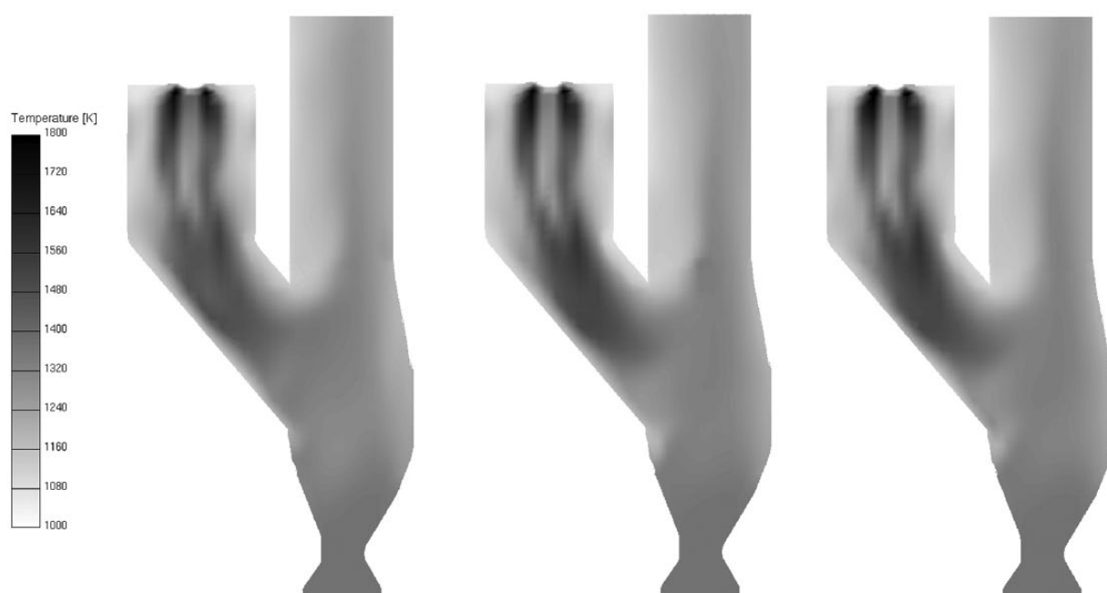
Figure 2. Temperature field inside the calciner: Case 1 (left); Case 2 (middle); Case 3 (right).
