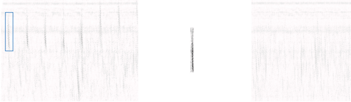
Fig. 1. An example of a B-scan (left) from which we extracted the defect patch (with a blue bounding box), a magnified extracted defect (middle), and an example of a UT B-scan without a defect.
