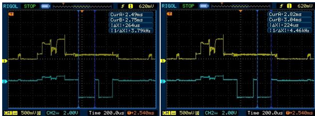
Figure 4-7 Time necessary to execute 64 bit division on nRF51 family microcontroller.
