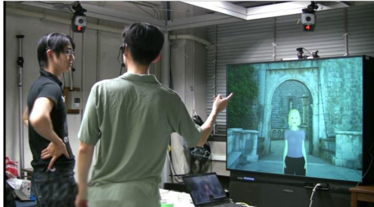
Figure 34: Detecting the situation in which users start speaking to each other
