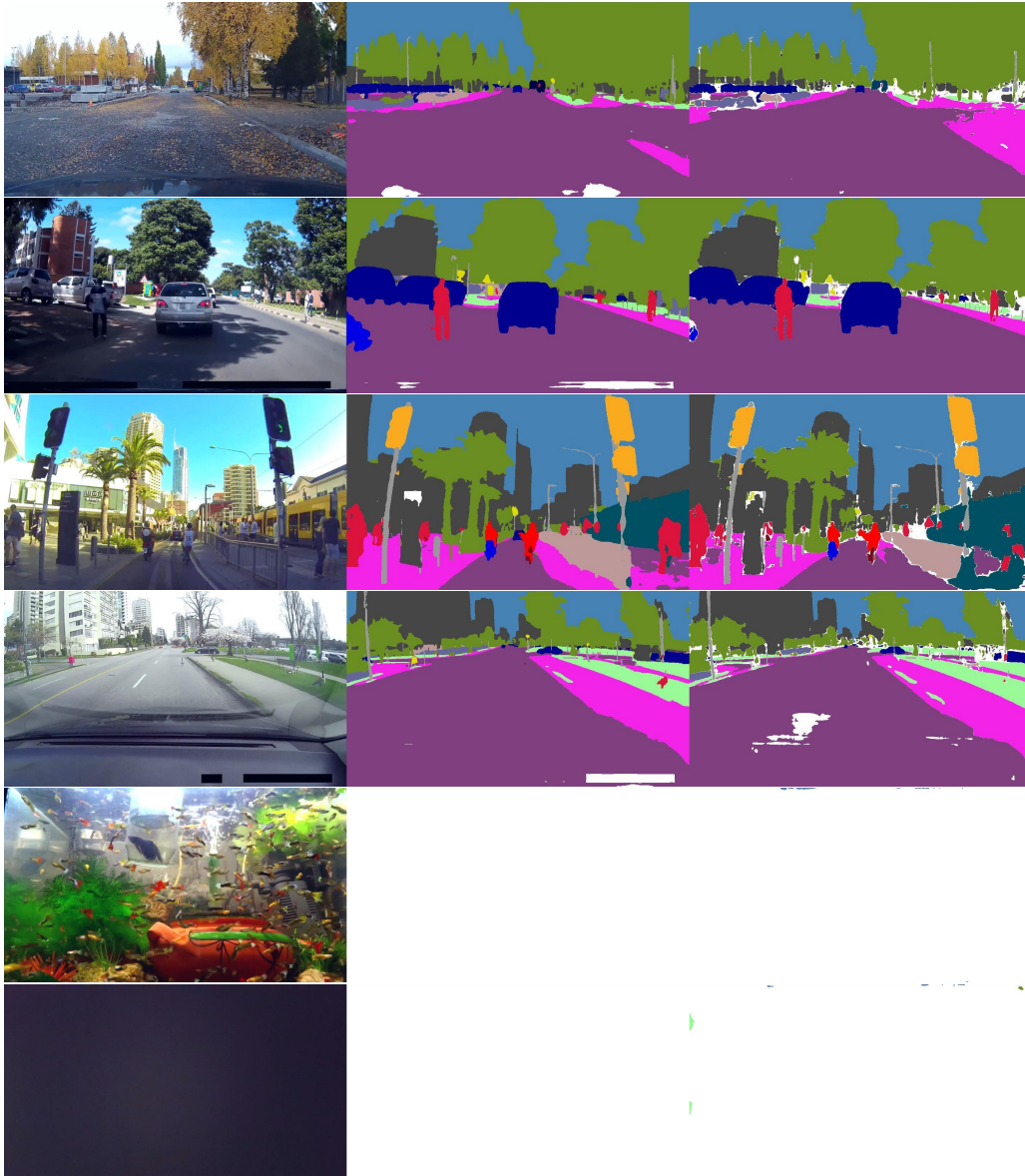
Figure 5.13: Qualitative performance on the WildDash benchmark. Each triplet contains a test image (left), the output of the two-head model (center), and the output of the C-way multi-class model trained to predict uniform distribution in outliers (right). The two-head model does not produce false positives at semantic borders (rows 1-4). Both models correctly recognize outliers in negative images (rows 5-6).
