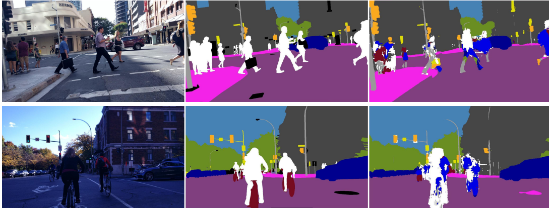
Figure 5.11: Open-set segmentation on Vistas-NP. The first column is the original image, the second the ground truth, and the third is the output of the two-head model that was trained with randomly sized pasted patches. Outliers are white while ignore pixels are black.
