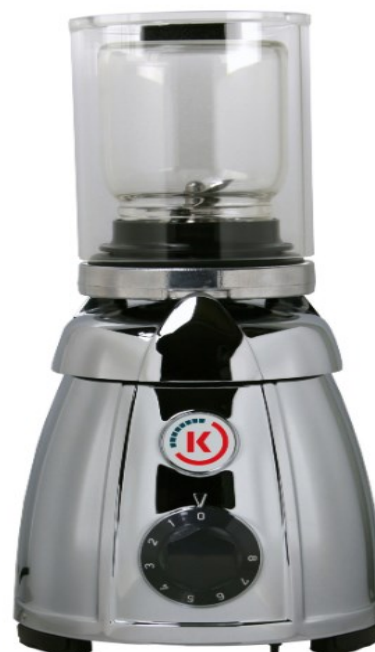
Figure 10. Microton MB 550 used for pulverizing flower heads of Dalmatian pyrethrum.
